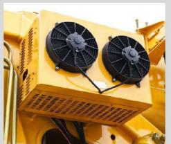
操纵室标配大功率制冷空调,提升空调制冷效果,可适应52℃以上高温环境。 High-power air conditioner is available in the operator's cab with improved cooling effect, which can endure high temperature environment of 52℃.
