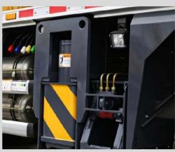
支腿作业灯夜间作业更安全 Outrigger working lamp makes night work safer
